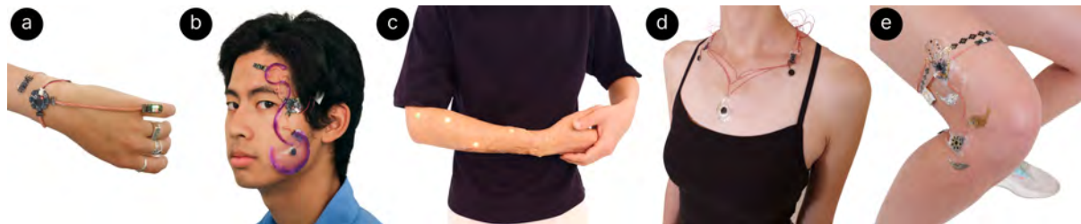
Fig. 1. SkinLink democratizes the design and prototyping of on-skin interfaces through linking, adjusting, and deploying customizable circuitry directly on the body. We designed a construction toolkit that contains skin-conformable circuit components for building slim and stretchable interfaces; an on-skin fabrication workflow allows experimenting with versatile device expressions. SkinLink enables the on-body fabrication of a minimalist on-skin interface (a), an expressive face circuitry (b), a concealed digital prosthetic (c), an infused smart skin jewelry (d), and an integrated sports training system (e).
