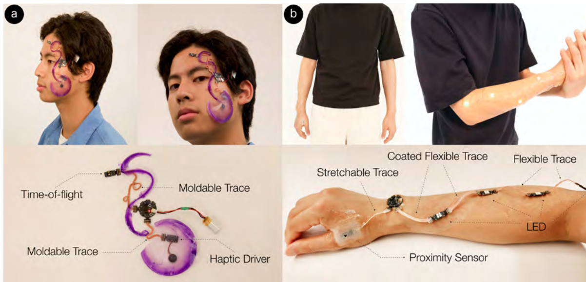
Fig. 13. (a) Victoria's project created a heartbeat on the cheek. She winded moldable trace modules to create intricate patterns paired with silicone prosthetics. The circuit consists of a time-of-flight sensor and a haptic driver. (b) Madison's project hid a proximity alarm on the forearm. She used a skin-tone foundation to camouflage the circuit with a thin layer of prosthetic skin. Four LED modules will light up gradually when the proximity sensor detects an object getting closer.
