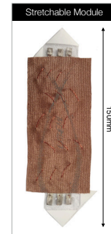
Fig. 5. The stretchable module is made of stretchable Kinesio tape. 3 insulated copper wires are sewn in a serpentine pattern to conduct current without obstructing the stretchiness.
