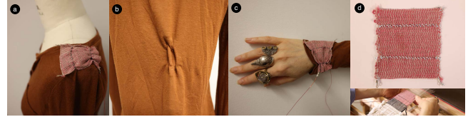
Figure 12: Blair's shrinking patch for form-fitting clothes, where she deployed on (a) the shoulder, (b) the back, and (c) the sleeve for a tailored effect. (d) The patch uses the Shrinking Primitive, with SMA coils integrated in the weft direction into a 2x2 twill weave.
