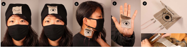
Figure 10: Ren's expanding patch for "opening a third eye," which she deployed on (a) the front of a hat, (b) earrings, (c) palm of the hand. The patch was woven with the Expansion Primitive of a double cloth with pre-trained shape memory SMA as a VIAS through the two layers.
