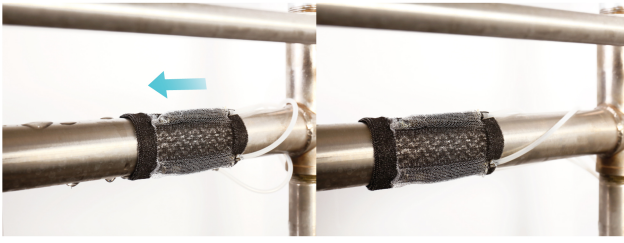
Figure 13: The KnitSkin ground layer can be knitted with a wide range of materials, including water soluble PVA yarn. When KnitSkin travels along a pipe and becomes exposed to water leaks, the PVA yarn dissolves and hardens as the yarn dehydrates. The hardened surface of KnitSkin could form a protective layer on the point of leakage.
